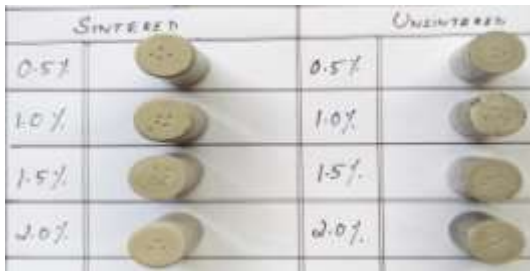
Fig.9 Samples of Mg/FA after RHN test
