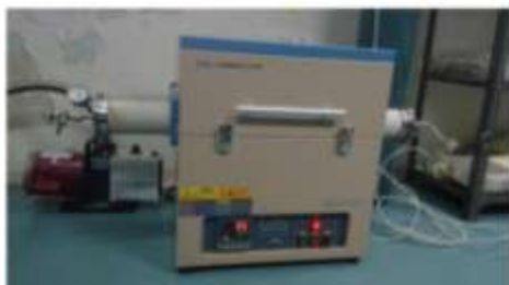
Fig.6 Vacuum Furnace Sintering
