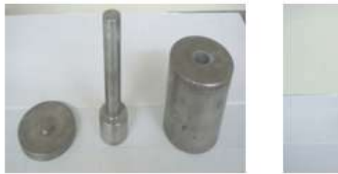
Fig.3 Disassembled & assembled parts of compaction die.
