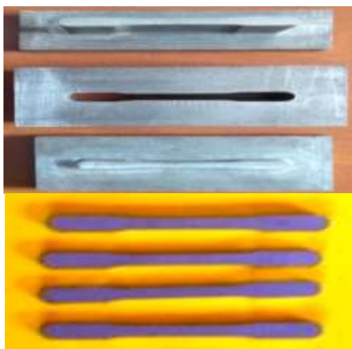
Fig.13 Standard flat Unmachined tension test specimen die as per ASTM & Specimens
