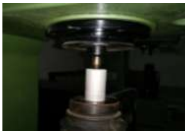
Fig.8 Sample for RHN test
